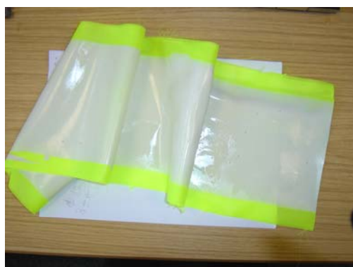
Figure 16. The manufacture of anti-Antibacterial PVA hydro gels with \text{TiO}_2 on the fabrics.
