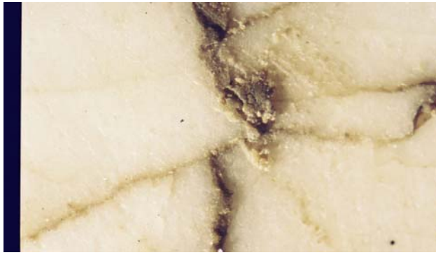
Figure 8. Cracks occurring on the surface after weight drop (brown powder is placed on cracks in order to make them more visible).
