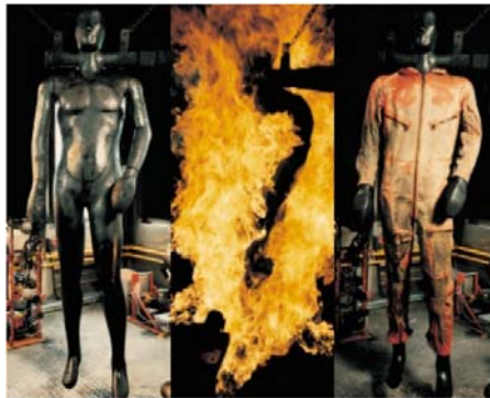
Figure 3. A view of a flame- retardant Nomex fabric's flammability test [5]
