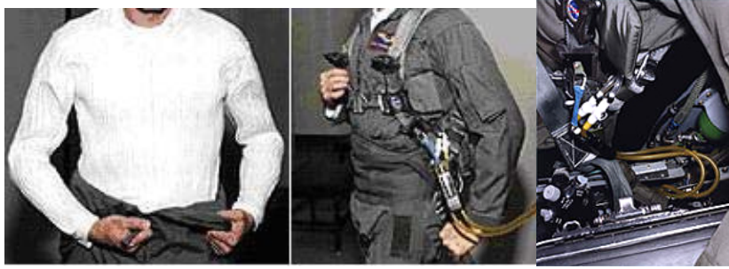
Figure 3. Liquid cooling vest for pilots (left), cooling garment connected to aircraft environmental system (right) [14]
