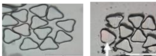
Figure 4. Optical transmission microscope images of transverse sectioned Ppy-pTSA coated Nylon-Lycra with different polymerization times: 60 min (a), 90 min (b), 120 min (c) and 180 min (d). Scale bar = 50 \mu\text{m} .
