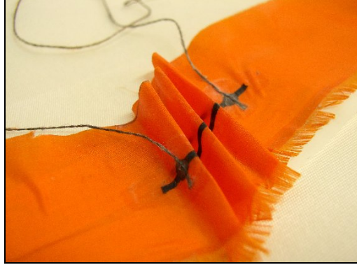
Figure 2. Set-up of sensor on fabric, with electrical connections
