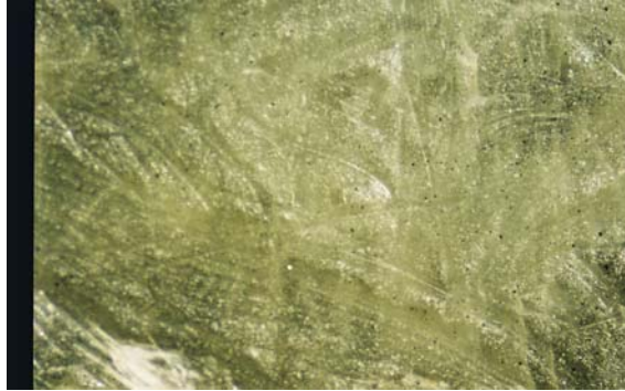
Figure 2. The air voids between the fibers of the composite plate produced by hand lay-up method and resin-rich regions.
