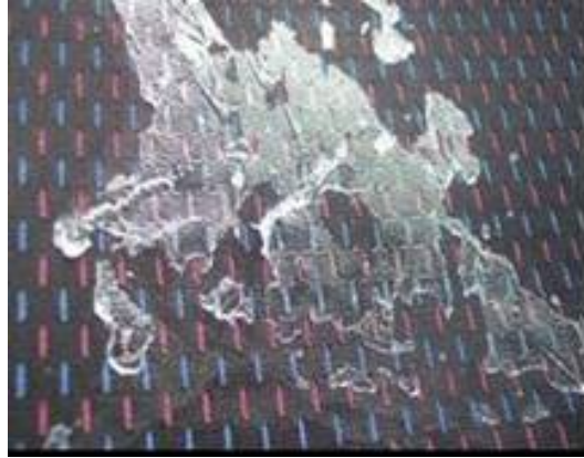
Figure 1: An image of the sticking problem between the upholstery fabric and the package film
