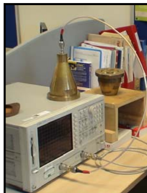
Figure 3. Coaxial test fixture relating to ASTM D 4935
