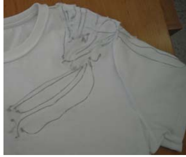
Figure 5. Conductive threads and connections in the inner side of the prototype
