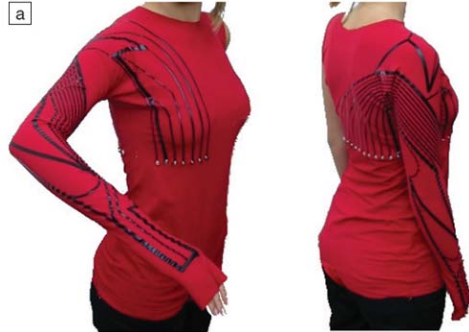
Figure 1. (a) Carbon-loaded elastomer-sensorized garment for kinesthetic monitoring developed at the University of Pisa.
