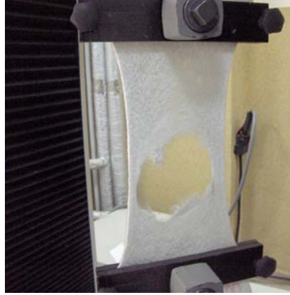
Figure 6 Deformation of fabric (500gr/m 2 ) in uniaxial tensile tests
