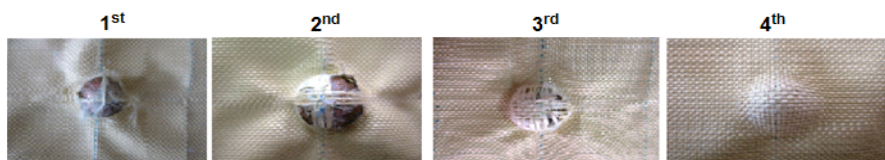
Figure 8. Effect of Ia thread type seen in between layers on multilayered one directional stitched structure from Twaron CT® 716 fabric where back of the first layer (first); back of the second layer (second); back of the third layer (third); back of the fourth layer (fourth). Shooting place is 5.
