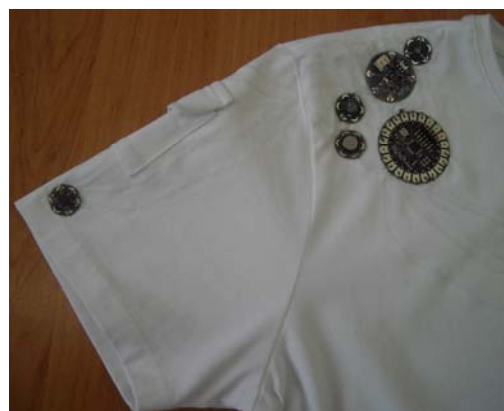
Figure 4. Modules on active t-shirt
