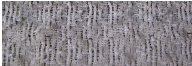
Figure 6: Weaving Fabric (warp:20/2 Ne Cotton, weft: 4 Nm stainless steel yarn, polyester fancy yarn)
