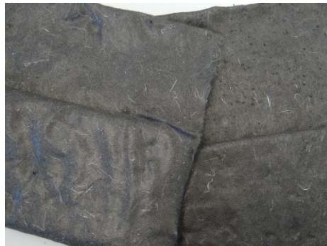
Figure 3. Wet-laid nonwoven made from production scrap
