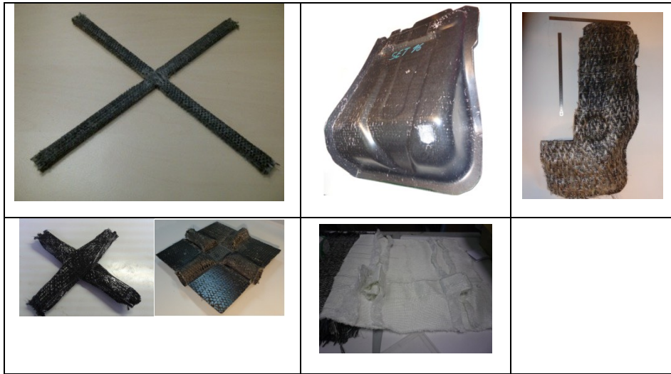
Figure 1. (1st column)(up) multiple woven cross stiffeners for railway application –(down)braided and 3D woven tubular cross for railway application – (2nd column) (up) 3D woven – (down) knitted seat frame for truck application – (3rd column) 3D woven automobile hood piece for automotive application.
