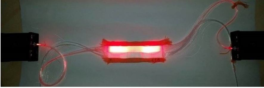
Figure 3. LEF sample connected to lasers by two ends
